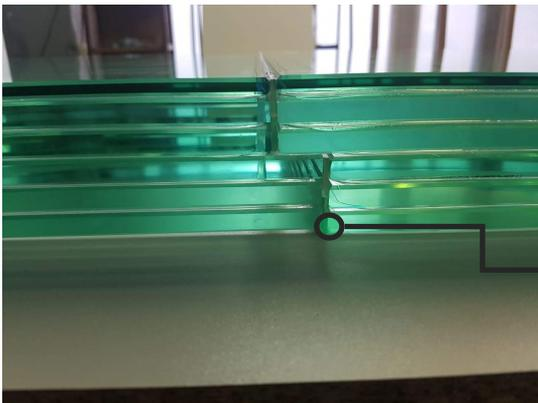
Zamil Frameless Bullet Proof Glass shall provides you endless view without intermediate frames, as well as providing Bullet resistance up to BR7 Level according to EN1063. Zamil provides Custom made Frameless Automatic Sliding Bullet Resistant Door also.
