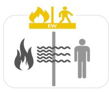
**EW - Integrity + Radiation Limit** Products to reduce radiant heat transfer (limit 15 KW/m<sup>2</sup> at 1m distance)
