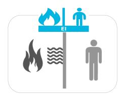
**EI - Integrity + Insulation** Products providing a barrier to radiant and conducted heat transfer (<140 °C)
